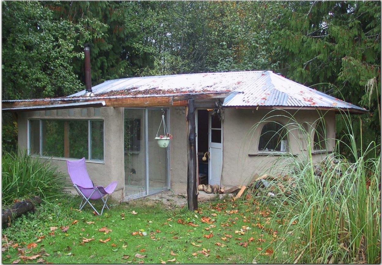
Patrick Loafman's art studio made of cob, which is clay, sand and straw.
